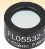
FL05532-1 Ø1/2" Filter CWL = 532 nm, FWHM = 1 nm
