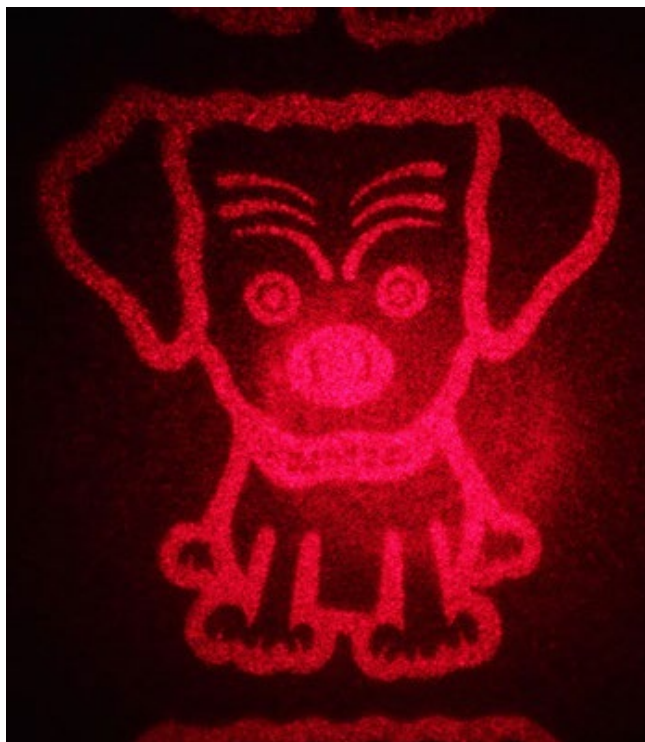
Figure 7: CGH projection of the CGH pattern shown in Figure 5 and the setup shown in Figure 6.
