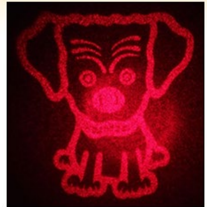
Image Generated by SLM Using Computer-Generated Hologram Projection. For Details, See the App Note Tab
