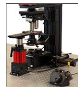
Click to Enlarge MCM3001 Being Used to Control Both Axes of the PLS-XY and a ZFM2020 Focusing Module
