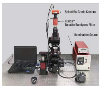
Click to Enlarge A hyperspectral imaging system built using Thorlabs' Cerna Microscopy Platform, KURIOS-VB1 Tunable Bandpass Filter, and Monochrome Scientific Camera. Several components shown here were modified from their stock configuration.
