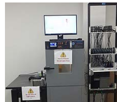
Enlarge Damp Heat Testing Setup
