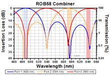
This plot shows an example of the spectral performance of a ROB58 ROB wavelength combiner. The lines represent the spectral response of each channel, while the colored regions denote the bandwidth around the center wavelengths. This data is typical; performance of each combiner may vary within the combiner specifications. Data was obtained without connectors.
