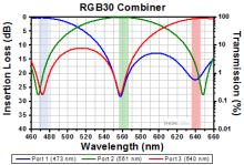
This plot shows an example of the spectral performance of a RGB30 RGB wavelength combiner. The lines represent the spectral response of each channel, while the colored regions denote the bandwidth around the center wavelengths. This data is typical; performance of each combiner may vary within the combiner specifications. Data was obtained without connectors.
