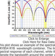
This plot shows an example of the spectral performance of a RYB54 RYB wavelength combiner. The lines represent the spectral response of each channel, while the colored regions denote the bandwidth around the center wavelengths. This data is typical; performance of each combiner may vary within the combiner specifications. Data was obtained without connectors.
