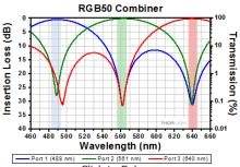
This plot shows an example of the spectral performance of a RGB50 RGB wavelength combiner. The lines represent the spectral response of each channel, while the colored regions denote the bandwidth around the center wavelengths. This data is typical; performance of each combiner may vary within the combiner specifications. Data was obtained without connectors.
