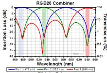
This plot shows an example of the spectral performance of a RGB26 RGB wavelength combiner. The lines represent the spectral response of each channel, while the colored regions denote the bandwidth around the center wavelengths. This data is typical; performance of each combiner may vary within the combiner specifications. Data was obtained without connectors.
