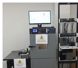
Click To Enlarge Damp Heat Testing Setup
