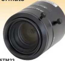
MVL25TM23 25 mm Fixed Focal Length, High Resolution (10 MP), 2/3" Format, C-Mount
