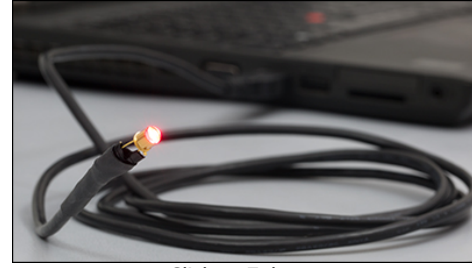
Click to Enlarge A LED630L being powered by the USB port in a laptop.
