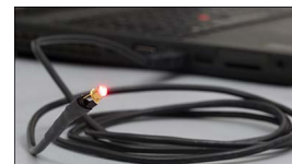
Click to Enlarge A LED630L being powered by the USB port in a laptop.
