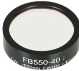
FB550-40 Ø1" Filter CWL = 550 nm, FWHM = 40 nm
