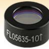
FL05635-10 Ø1/2" Filter CWL = 635 nm, FWHM = 10 nm
