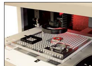
Click to Enlarge The front plate of a Polaris ® mirror mount is secured on the CMMP1212V within a vision system to verify its dimensions. Cap screws were used to secure and create stops for the parts being inspected.
