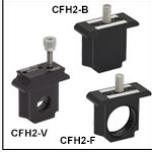
The CFH2(/M) Removable Filter Holder is a light-tight, stackable filter block designed to integrate easily into our 30 mm cage system or to be post mounted on a breadboard. Unlike the CFH1R above, this light-tight design is achieved with a permanent O-ring mounted on the front face and a double-flanged top plate on the removable inner body.
