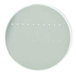
The photograph above is a protected aluminumcoated mirror after LIDT testing. In this particular test, it handled 0.43 J/cm² (1064 nm, 10 ns pulse, 10 Hz, Ø1.000 mm) before damage.
