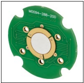
Click to Enlarge The Piezoelectric DM mounted on its circuit board. The three piezoelectric ceramic arms used for tip and tilt correction are seen around the edges of the mirror.
