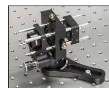
Click to Enlarge Figure 4: Spatial Filter System
