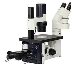
Click to Enlarge Multi-LED Source Coupled to Microscope Illumination Port
