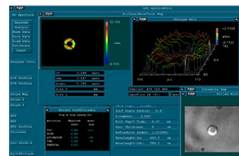
Click to Enlarge LMM40X-UVV Interferogram with Measured Seidel Coefficients
