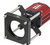
Click to Enlarge LCP4S Adapter Mounted to Quantalux® sCMOS Camera for Compatibility with 60 mm Cage Components. Note the LCP4S adapter has counterbored holes for 30 mm cage compatibility and through holes for 60 mm cage compatibility.
