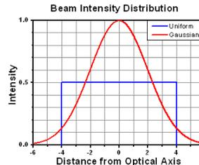
Thorlabs expresses LIDT for CW lasers as a linear power density measured in W/cm. In this regime, the LIDT given as a linear power density can be applied to any beam diameter; one does not need to compute an adjusted LIDT to adjust for changes in spot size, as demonstrated by the graph to the right. Average linear power density can be calculated using the equation below.
