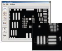
The screen captures to the right and left are actual measurements taken using a USAF 1951 resolution chart as the object.
