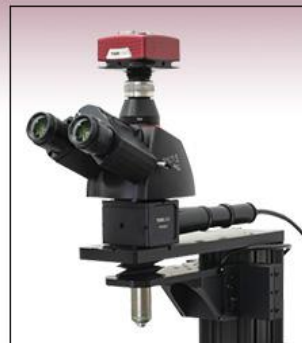
Application Idea 8051M-GE Scientific CCD Camera Mounted ®
