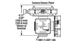
Click for Details Mechanical Diagram of the 2CM2 Double Camera Port
