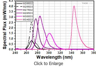
UV LED Spectra Scaled to Min Power
