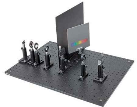
Click to Enlarge EDU-SPEA1/M Educational Kit Showing the Spectrum of a White Light LED Source
