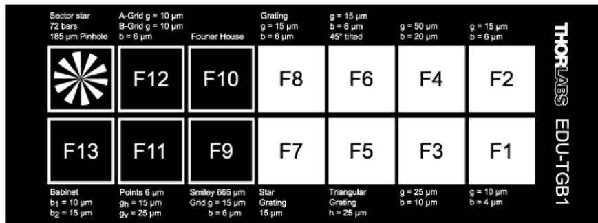
**Figure 3.** Diagram of Chrome-on-Glass Target Supplied with Fourier Optics Kit: Click on the numbered sections to see a detailed drawing of the pattern in each section. The white text along the edges of the slide is etched into the glass, but all other lines and dimensions shown in the detailed drawings are provided for reference only and do not appear on the actual slide. Black areas indicate chrome coating, and white areas indicate clear glass.
