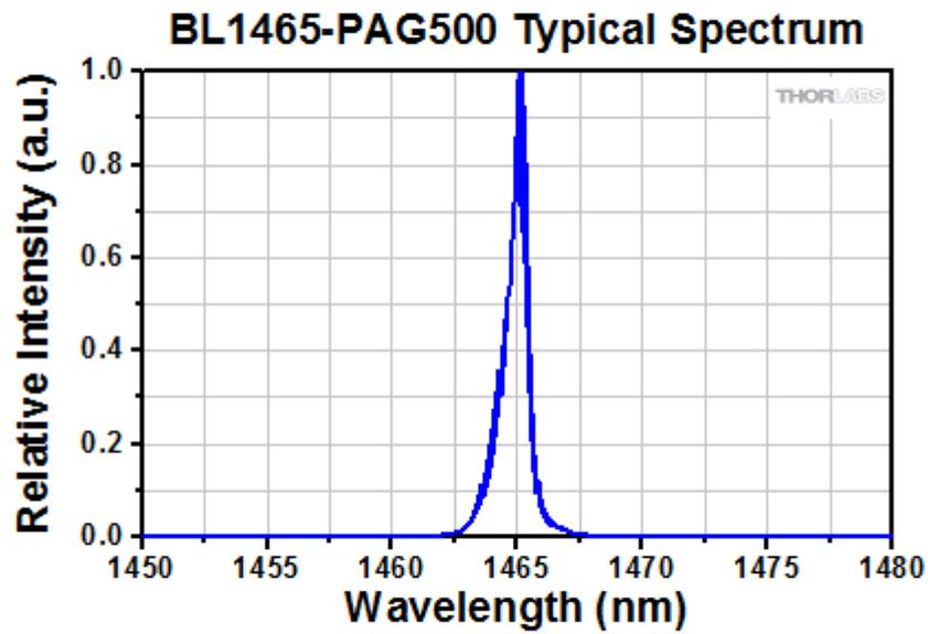
The typical optical spectrum is shown above. The laser diode was driven at  $P_{OP}$  (500 mW) and held at 25 °C. Performance will vary between individual lasers, serial-number-specific documentation is provided with each FBG-stabilized laser diode.
