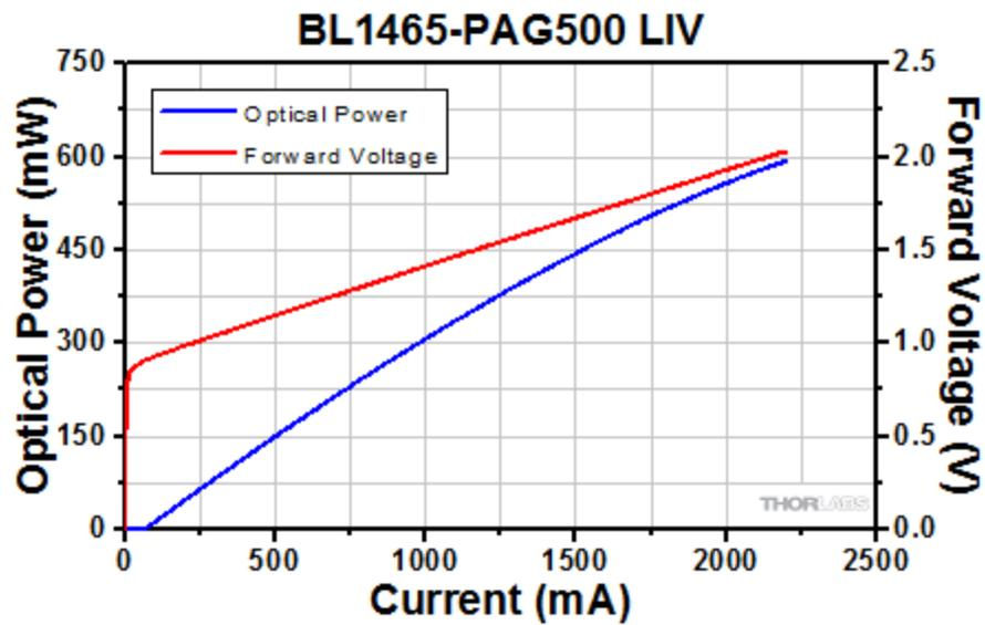
Note: The plot above is typical, and performance will vary between individual lasers. Serial-number-specific documentation is provided with each FBG-stabilized laser diode.
