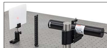
Click to Enlarge Light from a HeNe Laser Passing Through a Hole in a BHM1 Ruler
