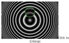
Figure 2: At left is shown a cross section of a ferrule with a polished fiber protruding from its ferrule. A representation of the interferogram created by this fiber can be seen to the right. In these images, the fiber end face is marked in green. Note how the
