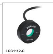
Thorlabs' Ø10 mm clear aperture, 3/4-wave liquid crystal retarder features an AR coating for 1050 - 1620 nm light. It has an outer diameter of 1", making it compatible with any of our Ø1" optic mounts for 8 mm thick optics. The RSP1 mount provides precise rotational adjustment and post mounting capability, while the CRM1P adds 30 mm cage-mounting versatility.
