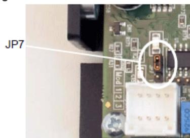
Servo driver cards manufactured after October 2009 have a jumper which is used to set the Volts per Degree scaling factor. The cards are shipped with the scaling set to 1.0 V/°, where the max scan angle is 10°, and is compatible with driver cards manufactured before October 2009.
