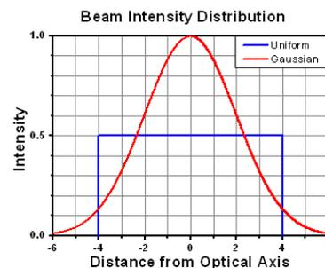
power density. For reference, a Gaussian beam typically has a maximum power density that is twice that of the uniform beam (see lower right).
