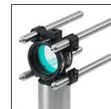
Click to Enlarge The CP02F(/M) Cage Plate offers a 1/4"-20 (M6) tap for mounting on our Ø1" Posts.
