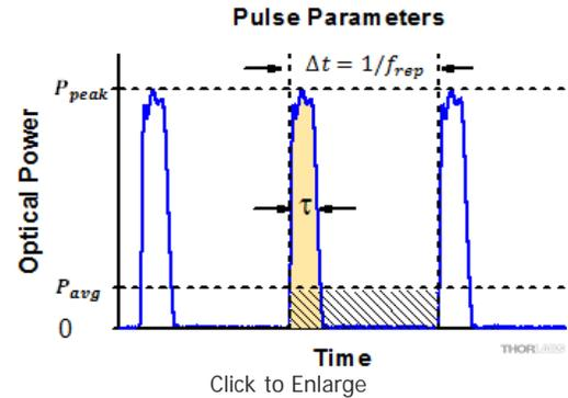
**Figure 1:** Parameters used to describe pulsed laser emission are indicated in the plot (above) and described in the table (below). **Pulse energy (E)** is the shaded area under the pulse curve. Pulse energy is, equivalently, the area of the diagonally hashed region.
