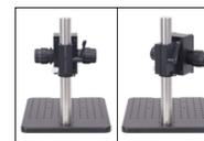
For convenient mounting of our Standard or User-Customizable Scanners, we offer a scanner stand that is ideal for use in vibration-sensitive studies such as angiography. It consists of a post-mounted focus block with knobs that provide both coarse (40 mm/rev) and fine (225 µm/rev) z-axis travel. A rotation and height collar underneath the focus block allows it to rotate 45° in order to move the scanner head away from the sample to make adjustments.
