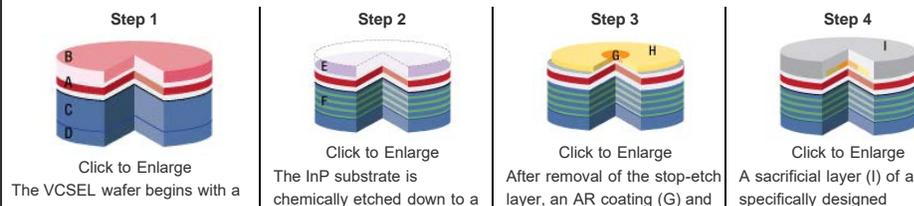
multiple quantum well (MQW) active region (A) that is grown on an InP substrate (B) and bonded to a GaAs-based mirror (C) grown on a GaAs substrate (D).
