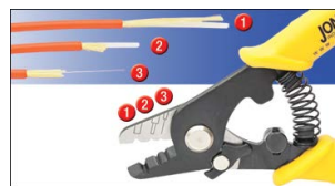
Click to Enlarge The FTS4 three-hole fiber stripping tool can be used to strip off (1) the jacket, (2) the buffer, and (3) the coating of an optical fiber.
