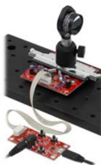
Click for Details [APPLIST] An ELL10K Linear Stage Bundle used to position a hollow roof mirror in an optical delay line.
