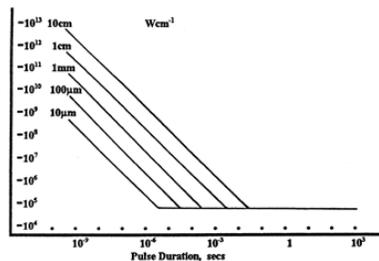
In order to use the specified CW damage threshold of an optic, it is necessary to know the following:
