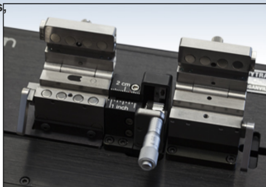
Close-Up View of the LDC400 Showing the Fiber Holding Blocks, Ruler for Cleave Alignment, and Micrometer Backstop
