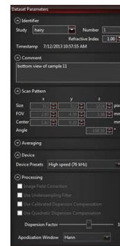
Click to Enlarge Various acquisition parameters can be adjusted in ThorImage OCT.
