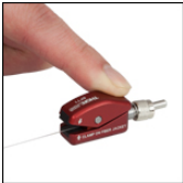
Click to Enlarge Step 4: Align Fiber Tip with Ferrule End
