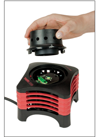
Figure 3: Lift the lens tube away from the LED housing.
