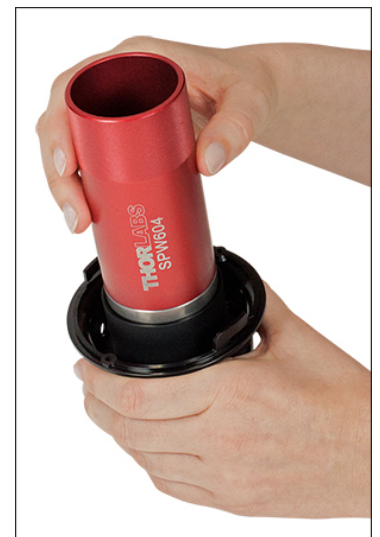
Figure 6: Use an SPW604 spanner wrench to lock the diffuser in place and re-install the lens tube onto the SOLIS housing by locking the bayonet mount in place and replacing the two screws.
