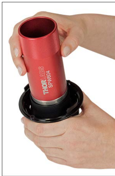
Figure 6: Use an SPW604 spanner wrench to lock the diffuser in place and re-install the lens tube onto the SOLIS housing by locking the bayonet mount in place and replacing the two screws.
