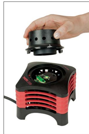
Click to Enlarge Figure 3: Lift the lens tube away from the LED housing.
