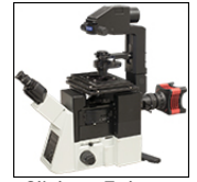
Click to Enlarge A Solis LED Installed on an Olympus Microscope
