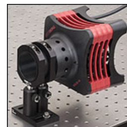
Click to Enlarge The SOLIS-1A shown mounted to an optical table using an SM2L15 lens tube, two SM2RC lens tube mounts, two Ø1/2" posts, and one BA2 post holder base.
