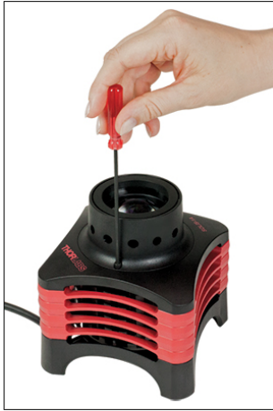
Figure 1: Remove the two screws holding the lens tube in place using a 2.5 mm hex key or balldriver.
