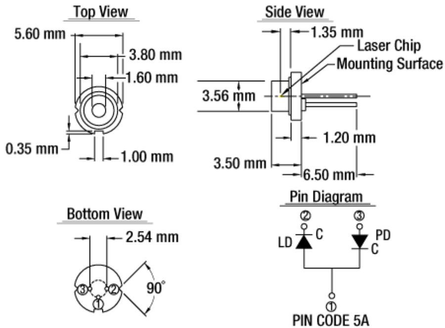
M5-905-0100 - 905 nm, 100 mW, Ø5.6 mm, A Pin Code, Laser Diode
