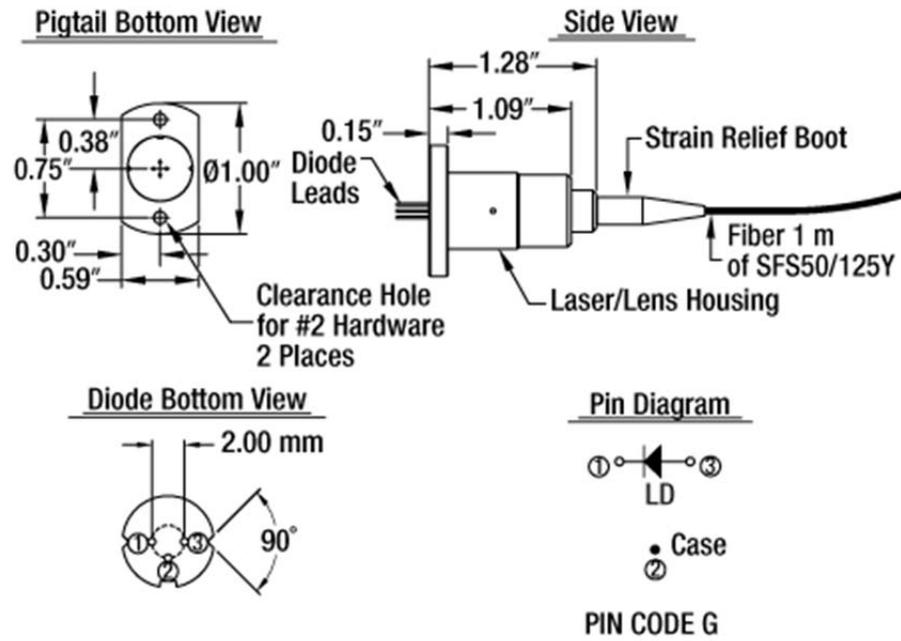
LP405-MF70 - 405 nm, 70 mW, G Pin Code,  $\varnothing 50 \mu\text{m}$  MM Fiber-Pigtail, FC/PC
