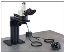
Click to Enlarge The MCM3000 3-Axis Controller, shown at the bottom right, is used to translate the objective focusing module along the Z-axis. (All items pictured here are sold separately.)
